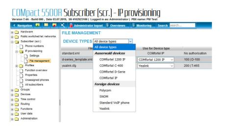
Once the telephone's MAC address has been connected to the internal subscriber, the PBX replaces the placeholders with the matching data, thereby creating a temporary provisioning file, and sends this file to the end device. It couldn't be simpler and saves the person performing the configuration lots of valuable working time.
